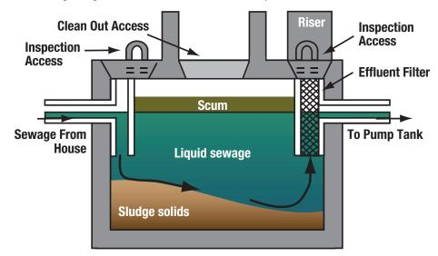
**CAUTION!!** Do not use septic tank additives with a low pressure pipe system. They allow partially broken down solids to be held in suspension and transported into the pump tank. This can cause a nasty gelatin-like substance to form in the pump tank, ruining the pump and clogging the lateral lines.
