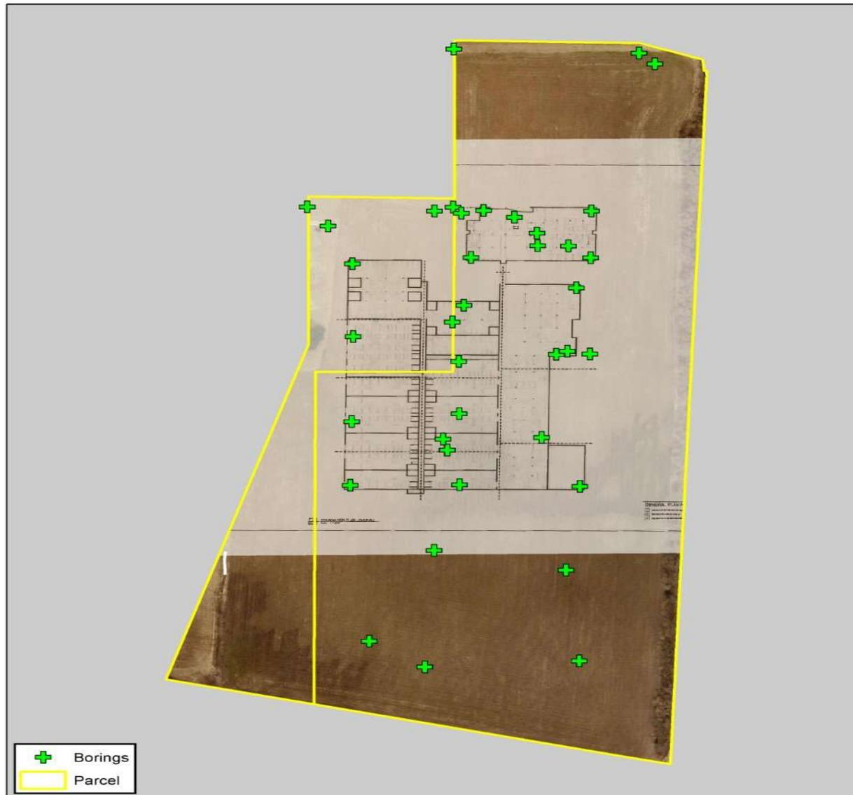
The green x's are locations of the drilled borings.
